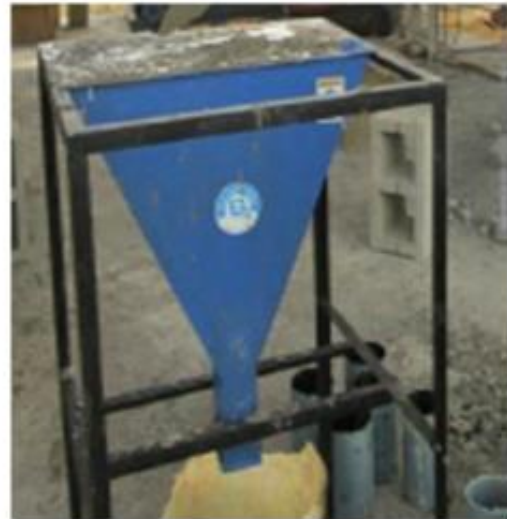
(b) V-funnel apparatus
