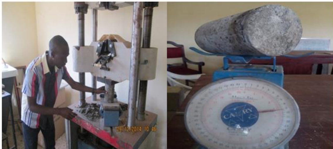
Figure 3: Compressive Strength Tests of Hardened Concrete Cylinders
